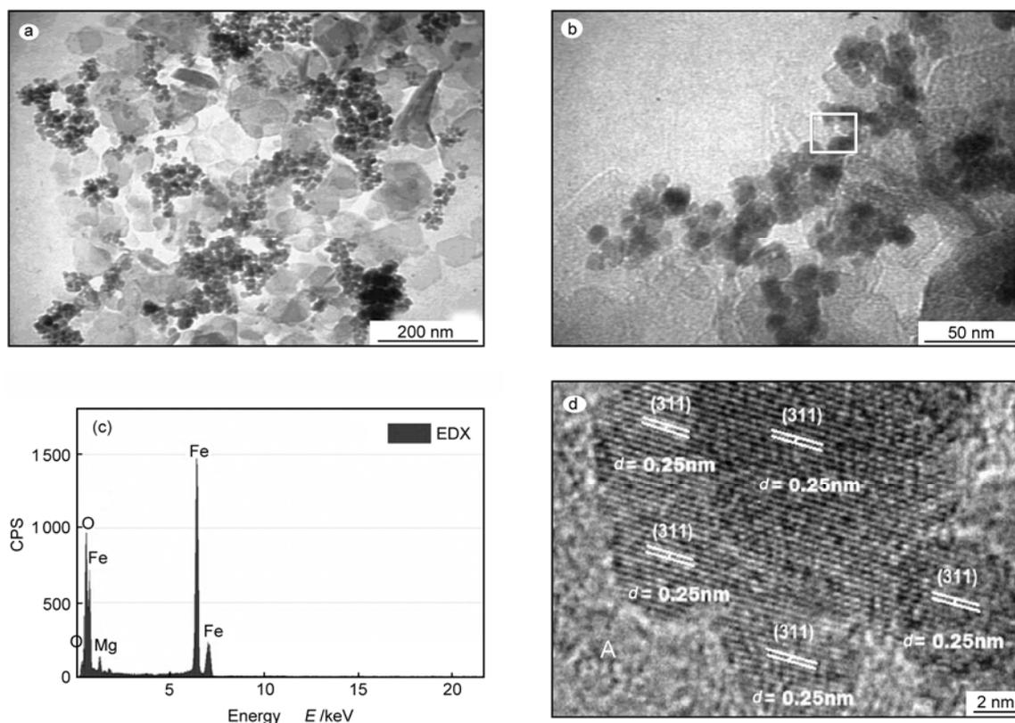
Fig.2 (a) Low-magnified and (b) high-magnified TEM images of  $\text{Fe}_3\text{O}_4$  nanoparticles supported on MgO. (c) EDX analysis of the  $\text{Fe}_3\text{O}_4/\text{MgO}$  catalyst. (d) HRTEM image of the  $\text{Fe}_3\text{O}_4/\text{MgO}$  catalyst
