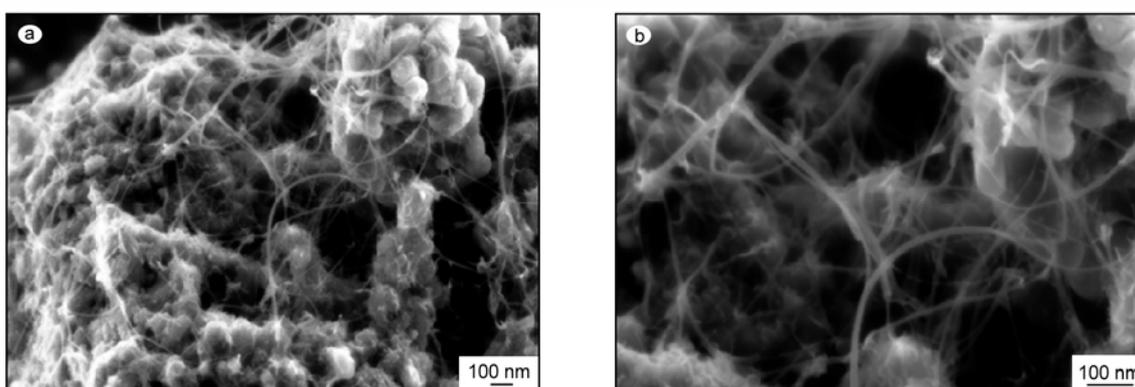
Fig.4 (a) Low-magnified and (b) high-magnified SEM images of the  $\text{Fe}_3\text{O}_4/\text{MgO}$  catalyst after methane decomposition
