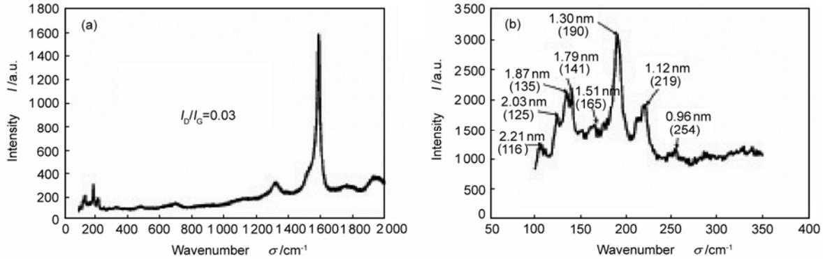
Fig.6 (a) Raman spectrum of SWCNTs. (b) The low-frequency region of Raman spectrum for the SWCNTs
