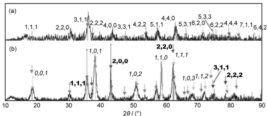
Fig.3 XRD patterns of (a)  $\text{Fe}_3\text{O}_4$  nanoparticles (b) the  $\text{Fe}_3\text{O}_4/\text{MgO}$  catalyst, (1,1,1): 01-075-0449(A)-Magnetite- $\text{Fe}_3\text{O}_4$ ; and (b) the  $\text{Fe}_3\text{O}_4/\text{MgO}$  catalyst, (1,1,1): 00-045-0946 (\*)-Periclase, syn-MgO, (1,1,1): 00-001-1169 (D)-Brucite- $\text{Mg}(\text{OH})_2$
