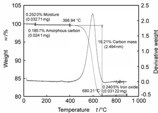
Fig.7 Thermal analysis of carbon sample
