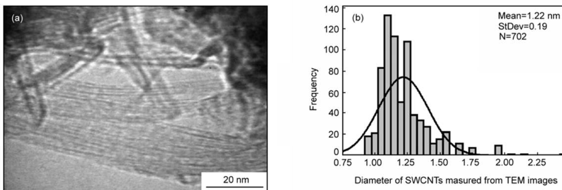
Fig.5 (a) TEM image of SWCNT bundles. (b) Diameter distributions of the SWCNTs
