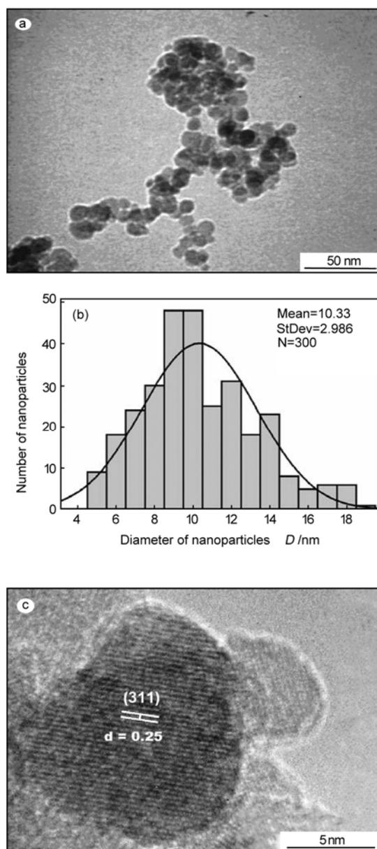
Fig.1 (a) Histogram showing the diameter distribution of  $\text{Fe}_3\text{O}_4$  nanoparticles. (b) TEM image of  $\text{Fe}_3\text{O}_4$  nanoparticles. (c) HRTEM image of  $\text{Fe}_3\text{O}_4$  nanoparticles.
