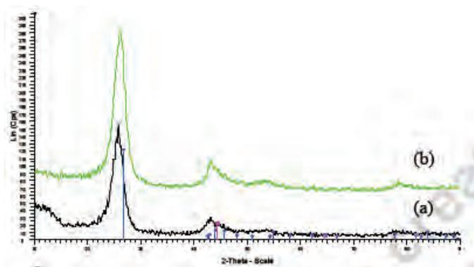
Fig. 1. X-ray diffraction patterns (Cu K $\alpha$ ) of (a) raw MWCNT and (b) functionalized MWCNT.
