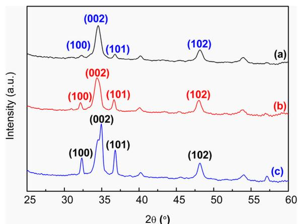
**Fig. 4.** XRD analysis ZnO-NPs thin films with different number of deposited layers via sol-gel and spin coating techniques. (a) 1, (b) 3, and (c) 5 deposited layers.
