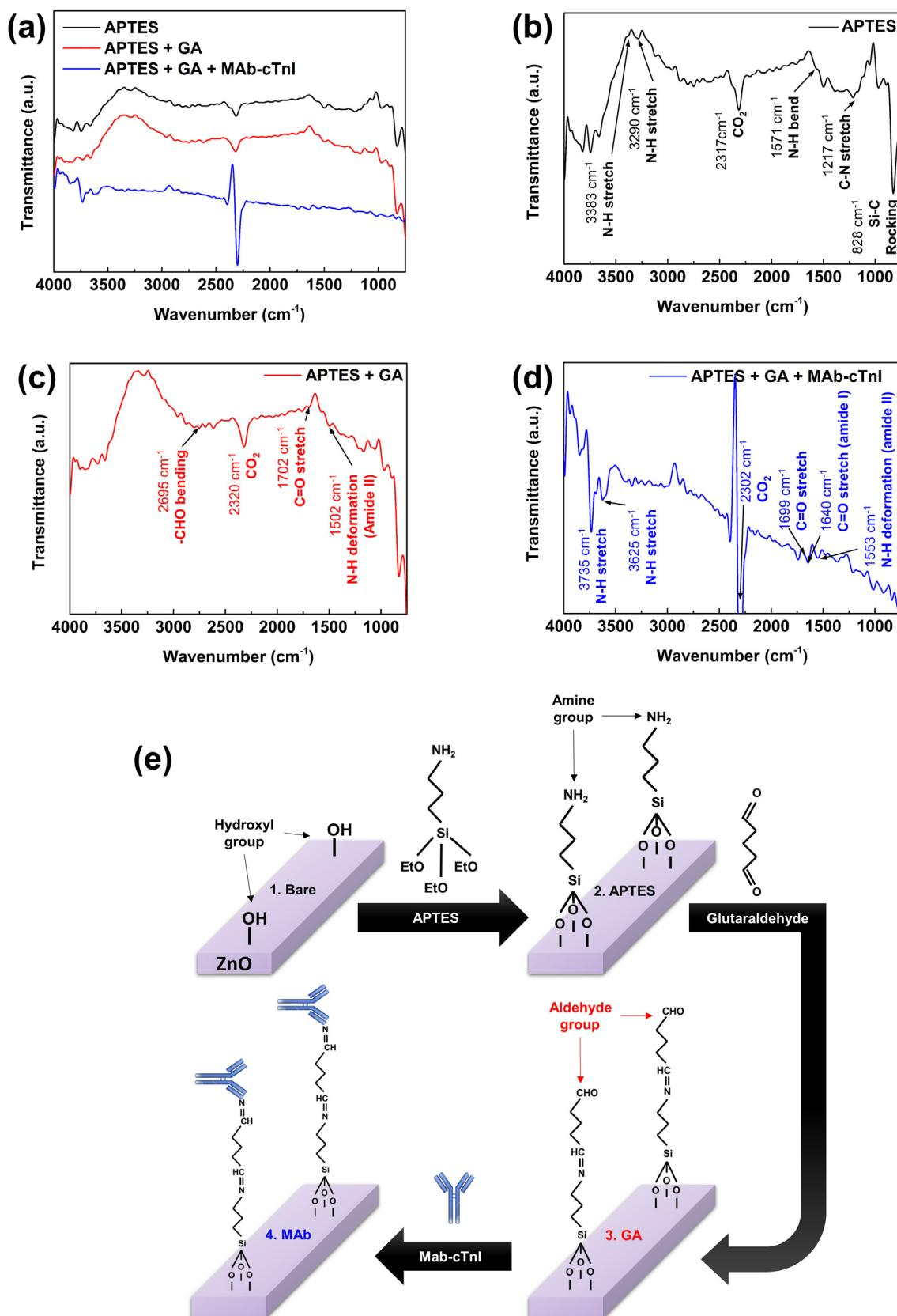
**Fig. 6.** Surface functionalization characterization of ZnO-NPs thin film. (a) FT-IR spectra adsorption of ZnO-NPs thin film deposited with (b) APTES, (c) GA, and (d) MAb-cTnI to functionalize the surface for capturing cTnI biomarker. (e) Overall stages of the surface functionalization on the thin film.
