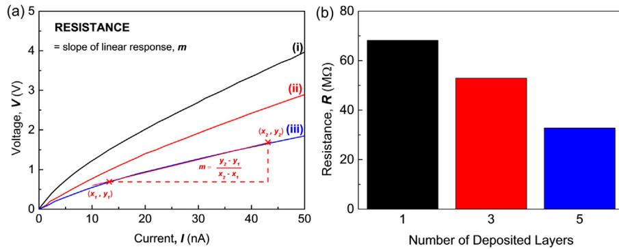
**Fig. 5.** Electrical characterization of ZnO-NPs thin films with different number of deposited layers via sol-gel and spin coating techniques. (a)  $V$  against  $I$  characteristic of (i) 1, (ii) 3, and (iii) 5 deposited layers. (b) Resistance histogram of the deposited thin film layers.
