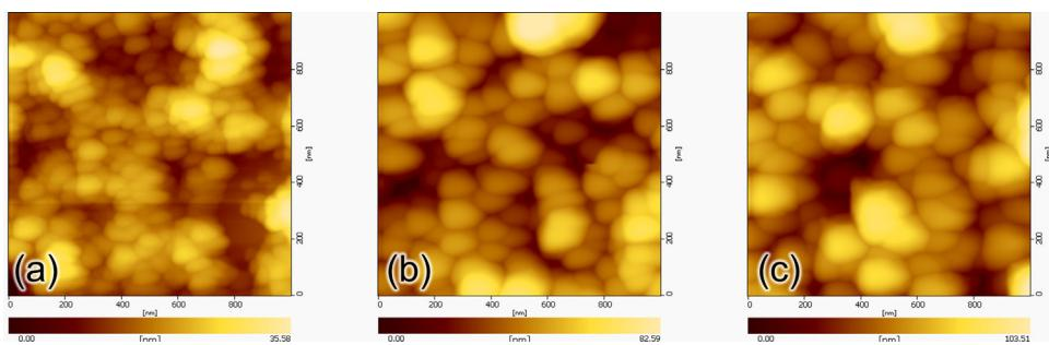
**Fig. 2.** 2D AFM characterization of ZnO-NPs thin films with different number of deposited layers via sol-gel and spin coating techniques. (a) 1, (b) 3, and (c) 5 deposited layers.
