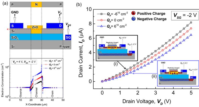
**Fig. 8.** Effect of extra charges introduced at the surface of the ZnO-NPs thin film as channel of the ZnO-FET biosensor with substrate-gate coupling. (a) Electron concentration along the cutline of the simulated 2D FET structure near the surface of the source, gate and drain region. (b) I<sub>D</sub> against V<sub>D</sub> characteristic of the biosensor with introduction of (i) negative and (ii) positive Q<sub>F</sub>.
