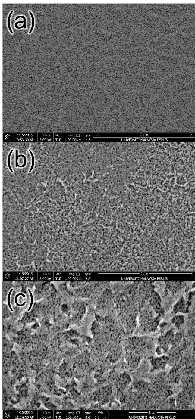
**Fig. 3.** FESEM images of ZnO-NPs thin films with different number of deposited layers via sol-gel and spin coating techniques. (a) 1, (b) 3, and (c) 5 deposited layers.
