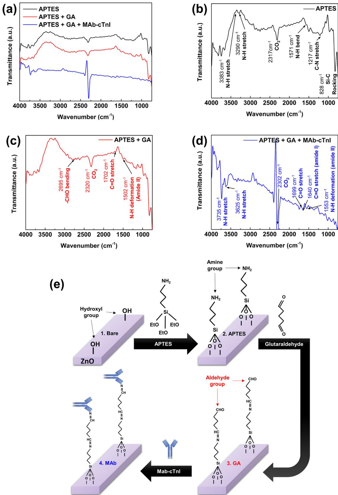
**Fig. 6.** Surface functionalization characterization of ZnO-NPs thin film. (a) FT-IR spectra adsorption of ZnO-NPs thin film deposited with (b) APTES, (c) GA, and (d) MAb-cTnl to functionalize the surface for capturing cTnl biomarker. (e) Overall stages of the surface functionalization on the thin film.
