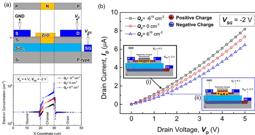
**Fig. 8.** Effect of extra charges introduced at the surface of the ZnO-NPs thin film as channel of the ZnO-FET biosensor with substrate-gate coupling. (a) Electron concentration along the cutline of the simulated 2D FET structure near the surface of the source, gate and drain region. (b) I<sub>D</sub> against V<sub>D</sub> characteristic of the biosensor with introduction of (i) negative and (ii) positive Q<sub>F</sub>.
