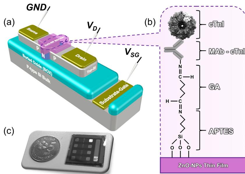
**Fig. 1.** Electrical detection of cTnI biomarker by ZnO-FET biosensor with substrate-gate coupling. (a) The 3D representation of the biosensor. (b) The surface functionalization of ZnO-NPs thin film with 3-aminopropyltriethoxysilane and glutaraldehyde; followed by surface immobilization process with cTnI monoclonal antibody for capturing cTnI biomarker. (c) The fabricated biosensor, comparable in size with Malaysia's 5 cent.
