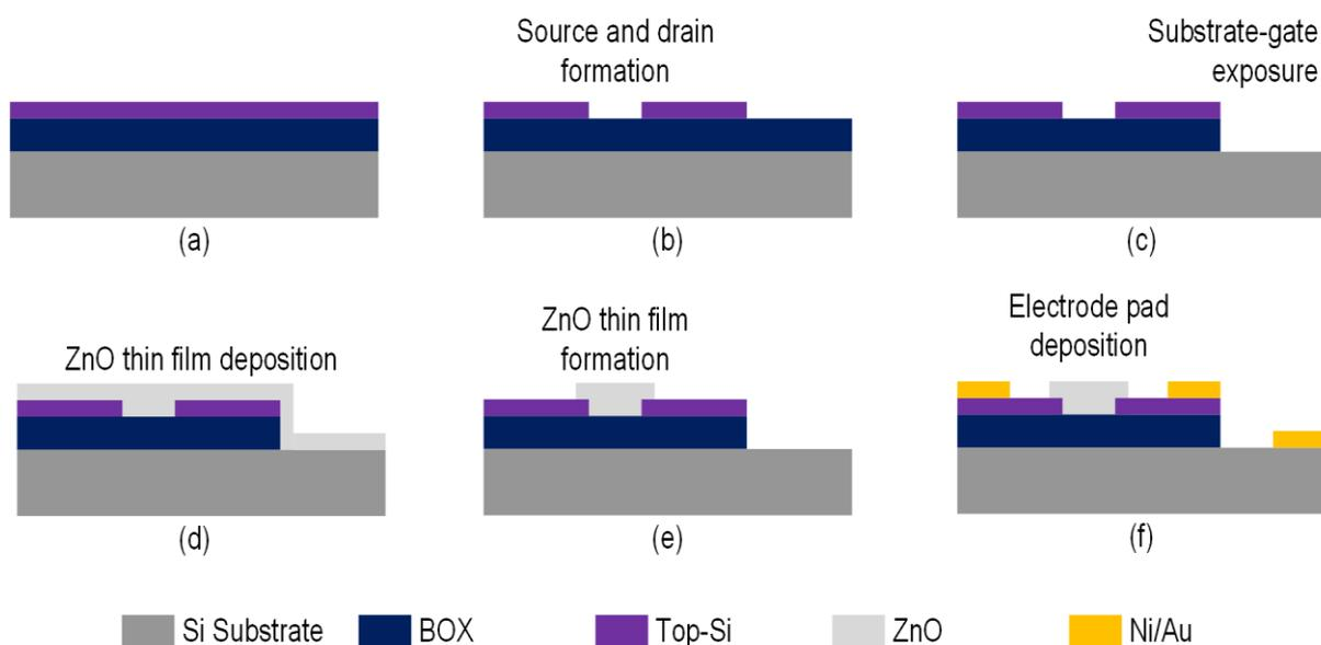
**Figure 3.** The fabrication process flow of ZnO-FET biosensor via conventional lithography processes. (a) Initial SOI substrate. (b) Source and drain formation via ICP-RIE of Top-Si. (c) Substrate-gate exposure by wet-etching of BOX layer. (d) Deposition of ZnO thin film. (e) Formation of ZnO thin film as channel by wet-etching. (f) Ni/Au deposition and formation as electrode pads.
