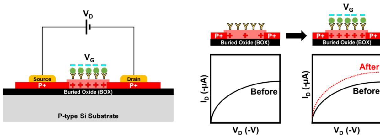
**Figure 2.** The architecture of the FET-based biosensor with the electrical characteristics during operation [9].
