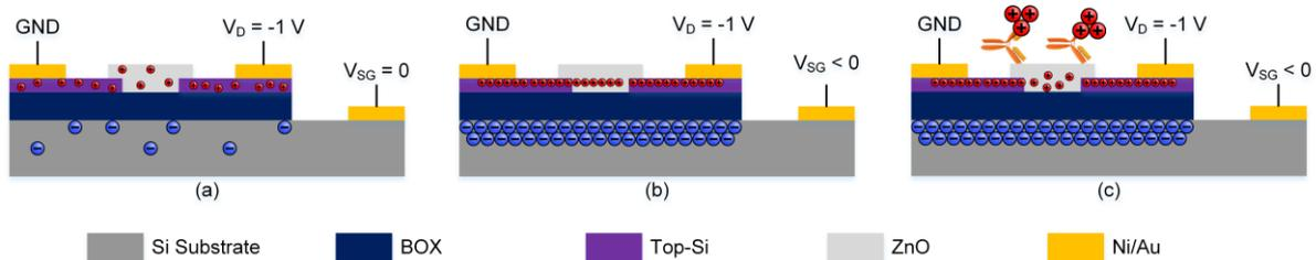
**Figure 7.** The impact of  $V_{SG}$  on the formation of hole conduction layer at the channel region. (a) Without  $V_{SG}$ , (b) With  $V_{SG} < 0$  V, and (c) during detection of positively charged cTnI target biomarker with  $V_{SG} < 0$  V.
