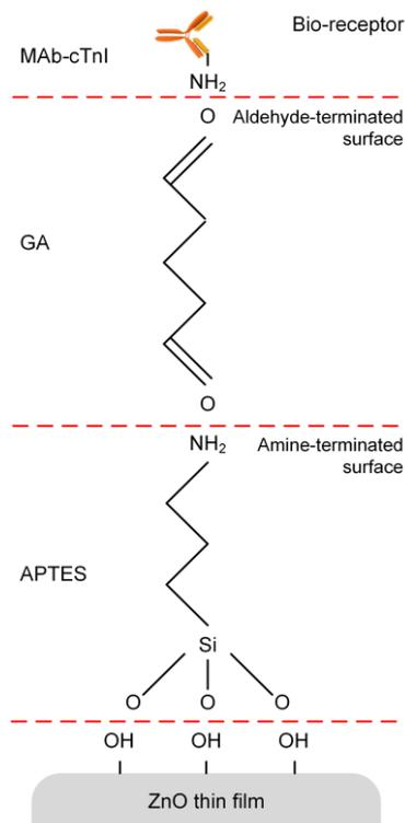
**Figure 4.** Surface modification of the ZnO thin film with chemical linkers (APTES and GA) and bio-receptor (MAb-cTnI).
