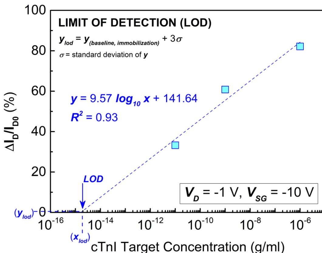
**Figure 10.** Limit of detection (LOD) of the ZnO-FET biosensor at  $V_{SG} = -10$  V and  $V_D = -1$  V.
