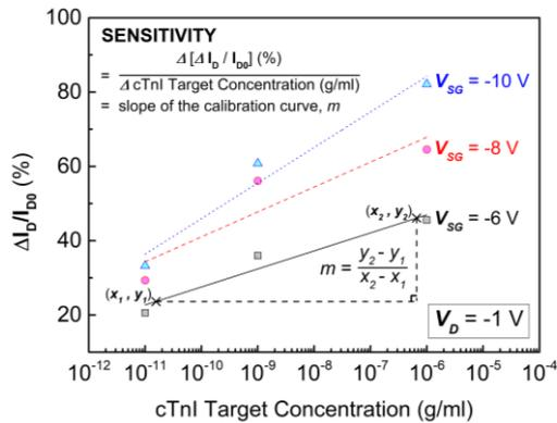
**Figure 8.** The sensitivity determination of the ZnO-FET biosensor at  $V_{SG} = -6, -8,$  and  $-10$  V. The relative change in  $I_D$  versus cTnI target biomarker concentrations.
