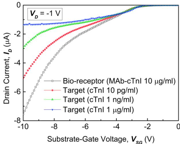
**Figure 6.**  $I_D$  versus  $V_{SG}$  of different cTnI target biomarker concentrations ranging from 10 p to 1  $\mu$ g/ml at  $V_D = -1$  V.
