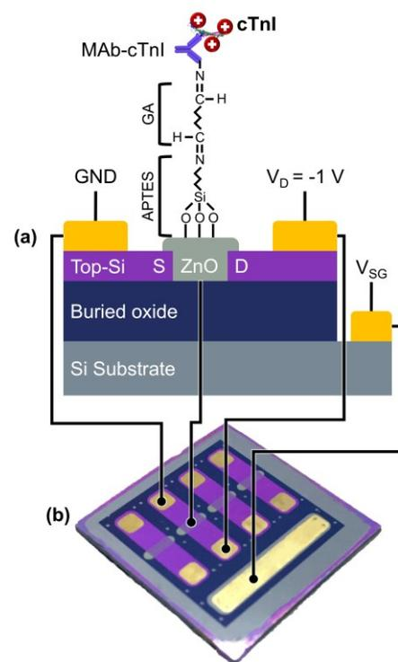
**Figure 5.** Device architecture of ZnO-FET biosensor. (a) Cross-section view of the device with surface modification. (b) The fabricated biosensor in array.
